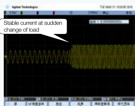
Current waveforms when sudden loading in vector control mode with 0.5Hz and full load
