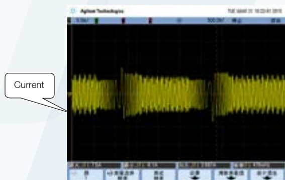
Current waveforms in vector control mode with 50Hz and full load
