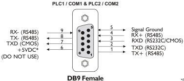
\*Do not use pin no. 6 of either of the GWY-00 communication ports.
