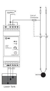
**Draining Control** (Single level Monitoring with two Sensors)
