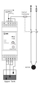
Filling Control (Single level Monitoring with two Sensors)
